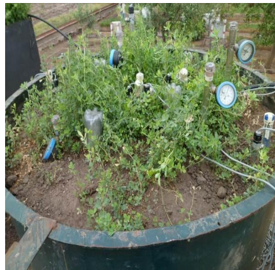
Figure 2. Lysimeter with alfalfa planted
