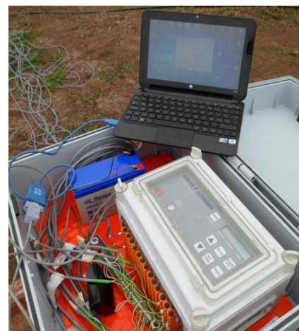
Figure 4. 40-cm-long tensiometer and data logger connected to the PC
