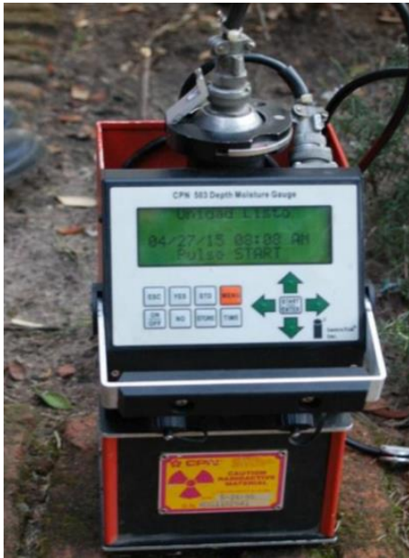
Figure 5. Neutron Probe model CPN 50
